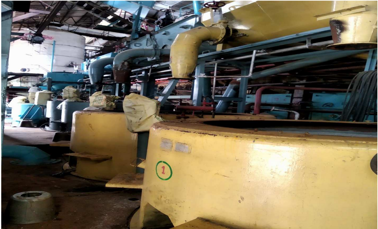
Batch Type machine – 1750 kg/charge capacity
