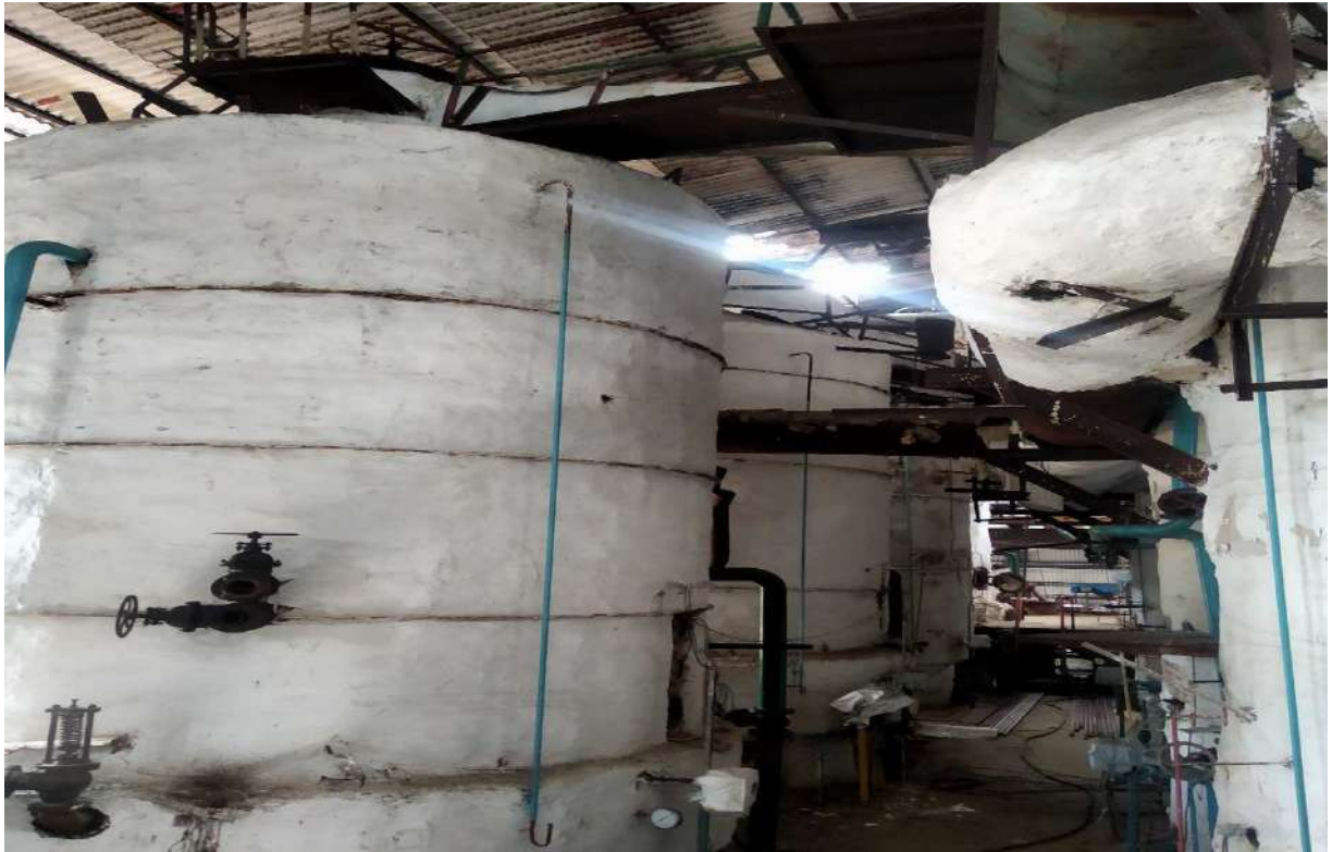
Pan Bodies 2 Nos ( 100 MT capacity each)
