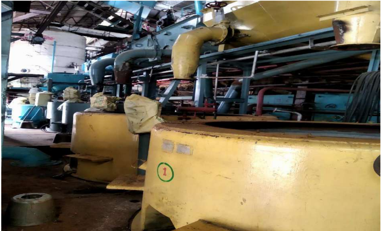
Batch Type machine – 1750 kg/charge capacity
