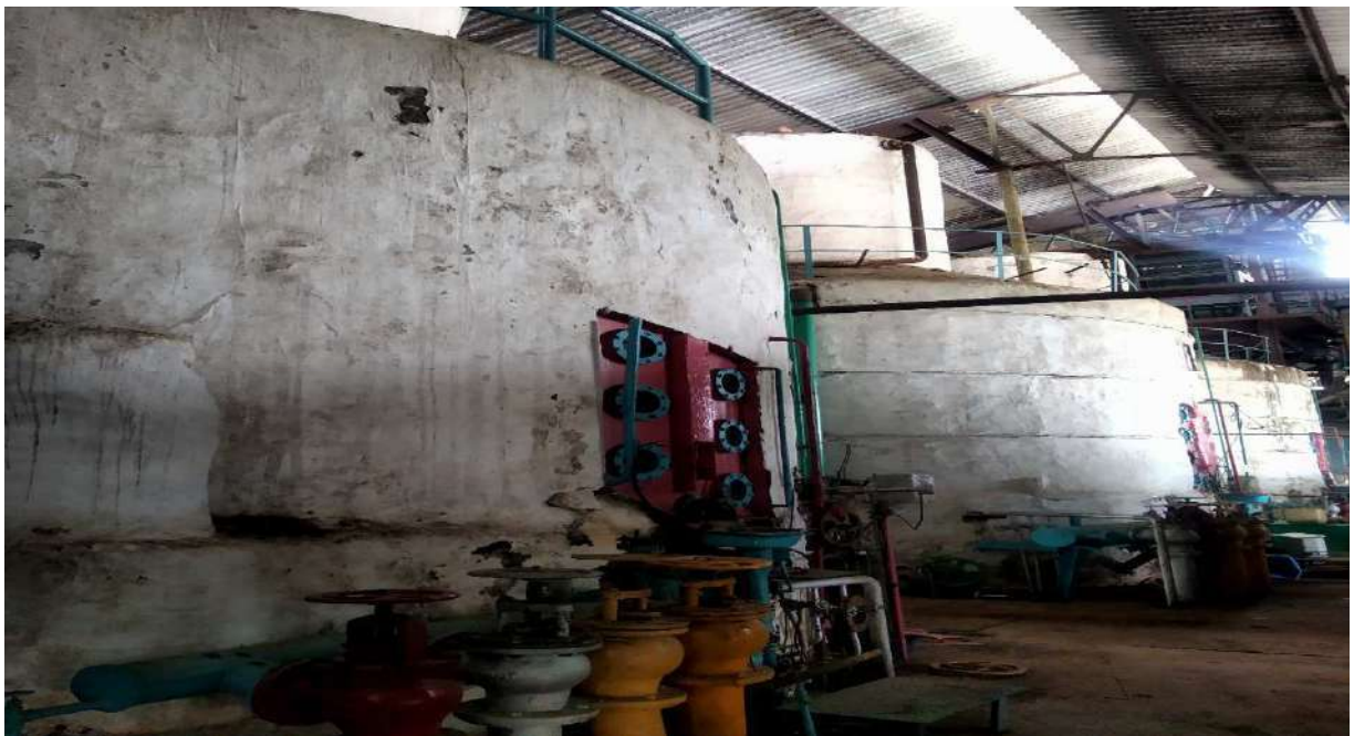
Pan Bodies 2 Nos ( 100 MT capacity each)
