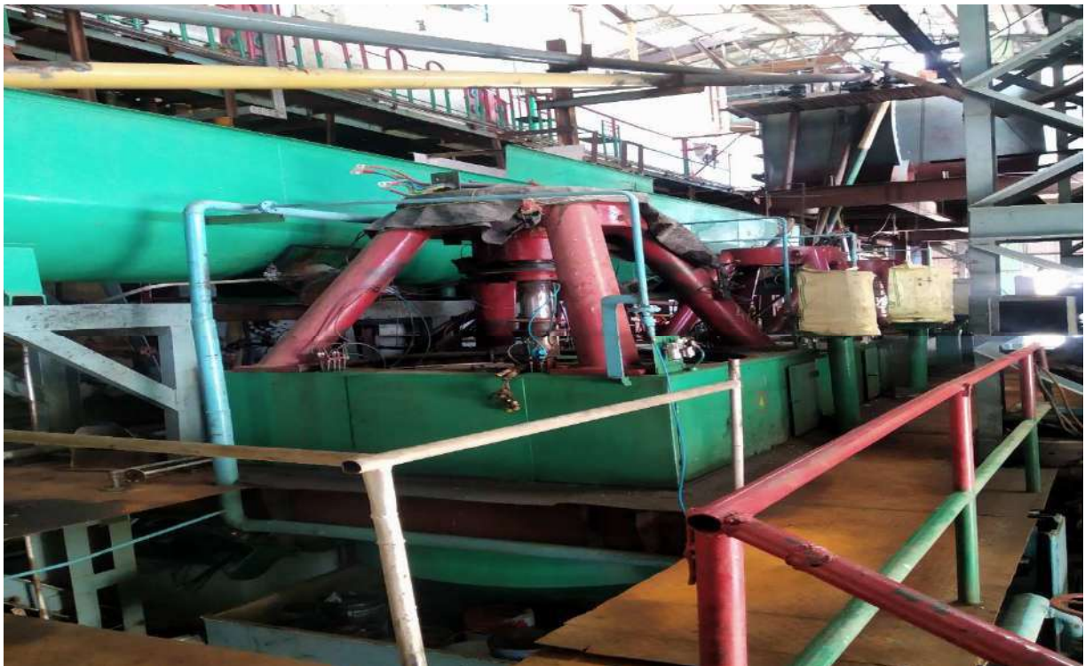
Batch Type machine – 1750 kg/charge capacity
