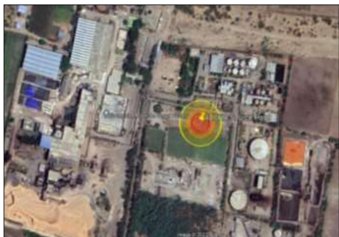
Figure 3.8: Thermal radiation threat zone mapping of SMSKL
